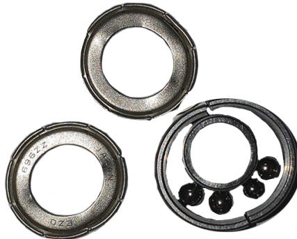
Figure 5.9: First attempt to damage a bearing in a controlled way. The end result was a crushed bearing.
