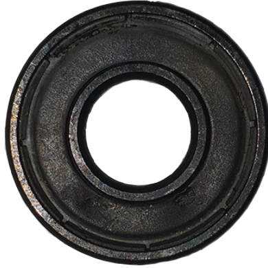
Figure 5.10: Bearing after damaging by blow torch and hitting with a hammer. It still has its shape but is severely blackened from the heating and burning of grease.
