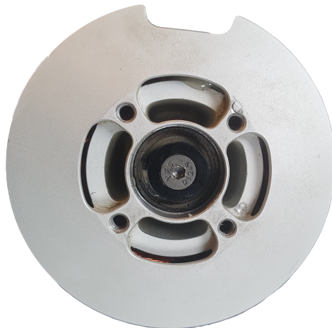
Figure 5.11: Under side of the MN505-S where the lower bearing has been replaced with a damaged bearing. One can see that the bearing is a damaged sample by the charring.
