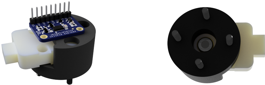
(a) Top view of the accelerometer and contact-less temperature sensor package.
