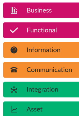
Figure 1.2: The architecture layers of the RAMI 4.0.
