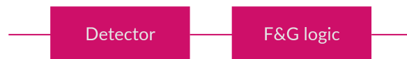
Figure 2.2: RBD for gas detection with one detector SIF, adapted from Offshore Norway, 2022.
