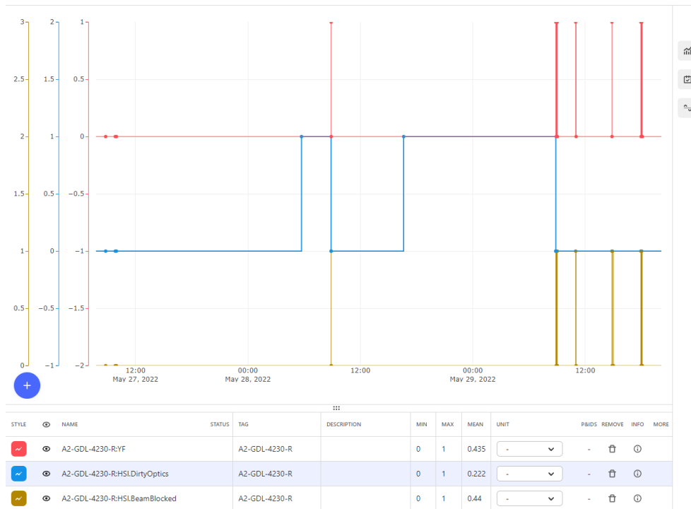
Figure 7.7: Dirty optics, beam block and fault in CDF charts.
