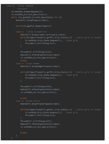
Figure 58: The case which controls the dropping sequence.
