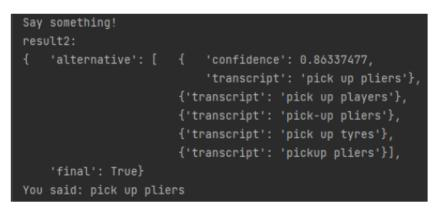
Figure 95: Correct recognition of pliers command
