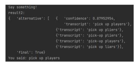
Figure 96: Incorrect recognition of pliers command
