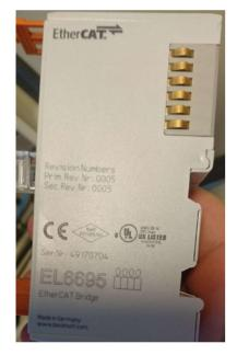
Figure 30: EtherCAT bridge module used in the project
