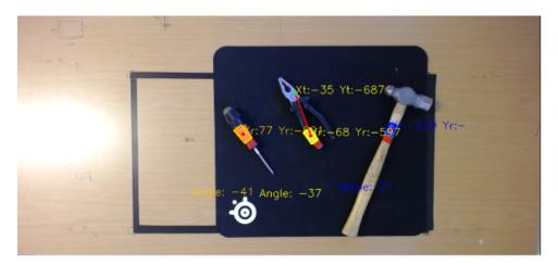
Figure 99: Example of tools recognized by webcamera using computer vision library "OpenCV"
