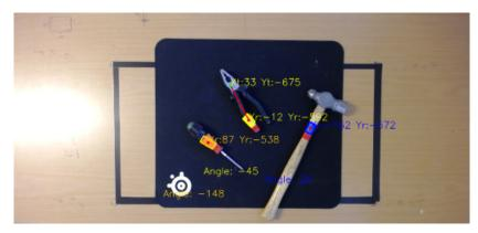
Figure 100: Example of computer vision application having difficulties to correctly calculate angle of screwdriver
