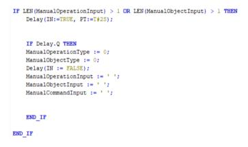
Figure 46: The reset logic of inputs and outputs within manual mode.
