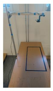
Figure 75: Camera stand made from aluminium profiles
