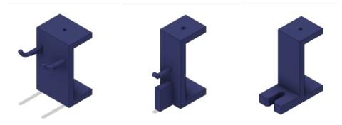
Figure 90: 3D models of the tool stands made in Fusion 360 software
