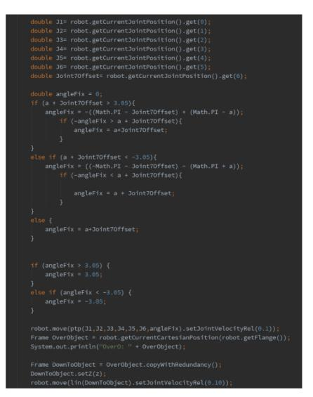
Figure 57: Angle transformation algorithm along with movements performed to prepare for object grasping.
