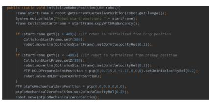
Figure 52: InitializeRobotPosition() method within RobotUtil class.
