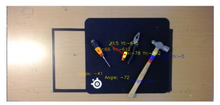
Figure 101: Example of computer vision application having difficulties to correctly calculate offset coordinates and angle for pliers
