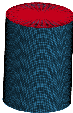
Figure 9.1: Tower with rotational motion creating bending moment.
