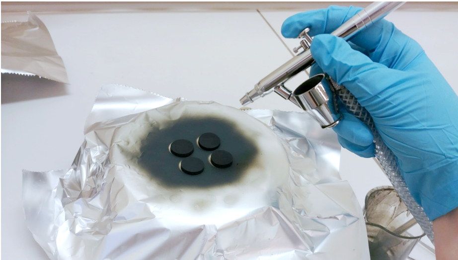
Figure 3.9: Spray coating of the suspension containing nanocrystalline [\text{Ho}_{0.98}\text{In}_{0.02}]_{0.97}\text{Mn}_{0.85}\text{Ti}_{0.15}\text{O}_3 powder on top of \text{Y}_{1.05}\text{Mn}_{0.85}\text{Ti}_{0.15}\text{O}_3 porous substrates.
