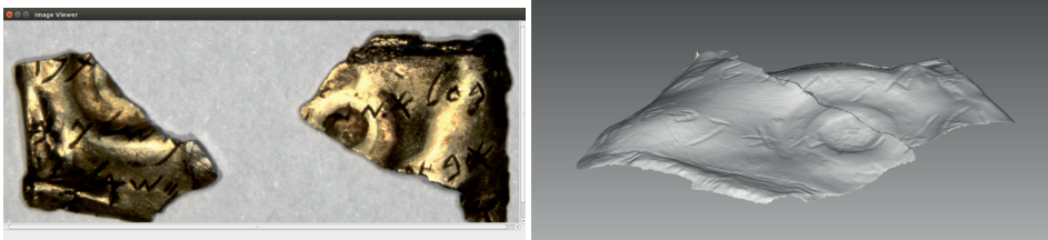
Figure 3.4: Left: The two fragments of the lamina relighted from a perpendicular light position, which is originally uncaptured, as it coincides with the camera position in the acquisition setup. Right: The virtual reassembly of the two fragments by visually matching shape clues.
