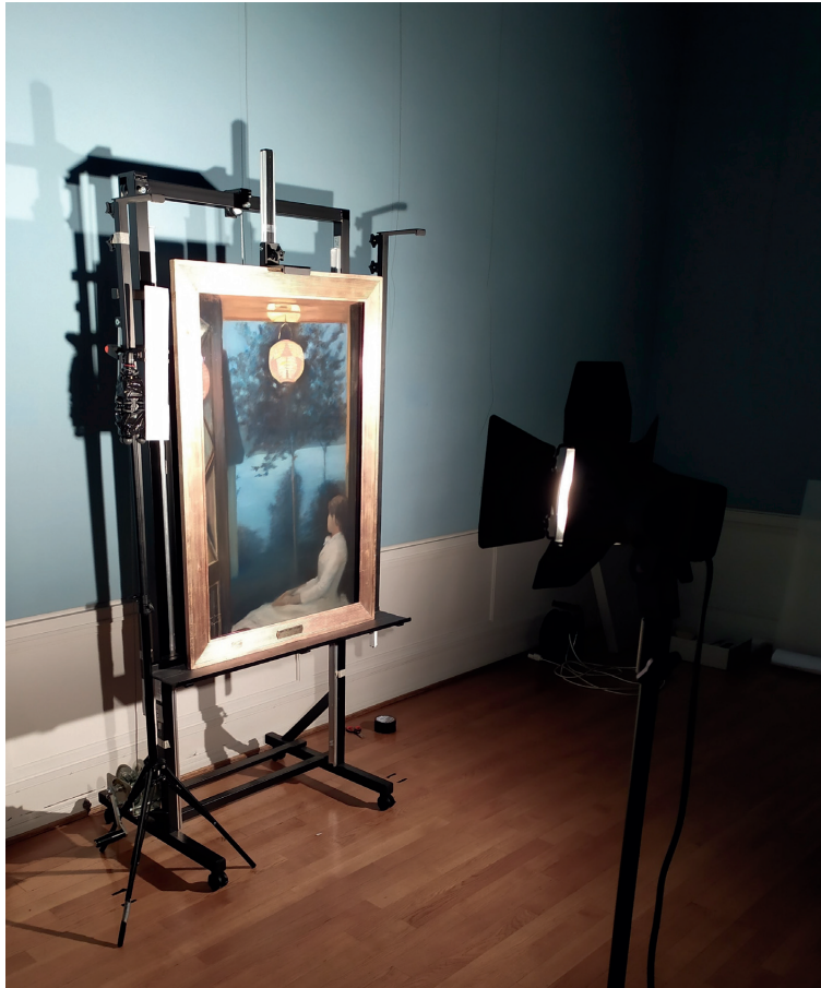
Figure 3.11: Setup for the in-situ hyperspectral image acquisition of the painting “A Japanese Lantern”.
