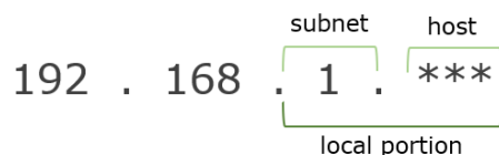
Figure 5: Division of an IP address' local portion
