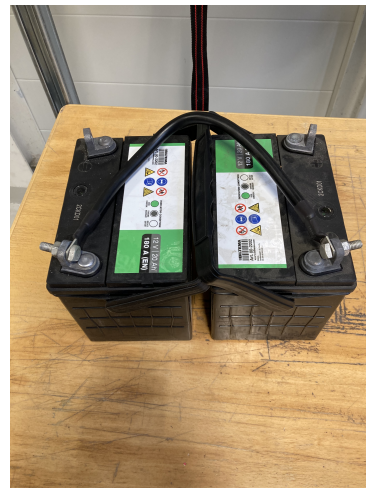
Figure 4.10: New 12V batteries used for electrical storage in the system.
