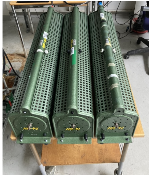
Figure 4.13: Three variable resistances used for demonstrating wind to heat.
