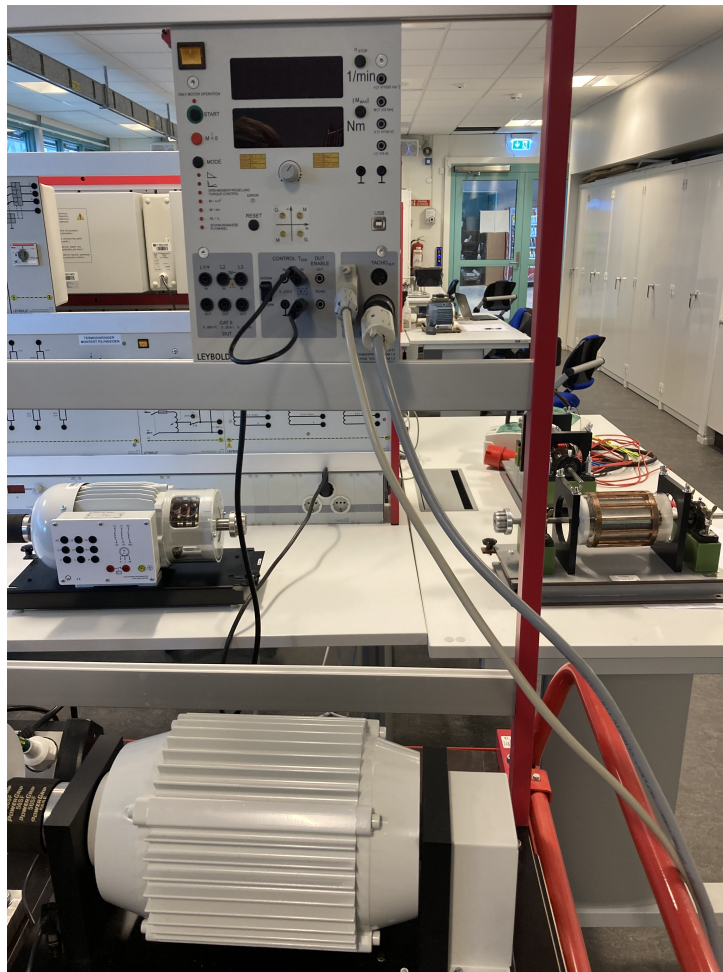
Figure 4.2: RPM controlled asynchronous machine with control unit.
