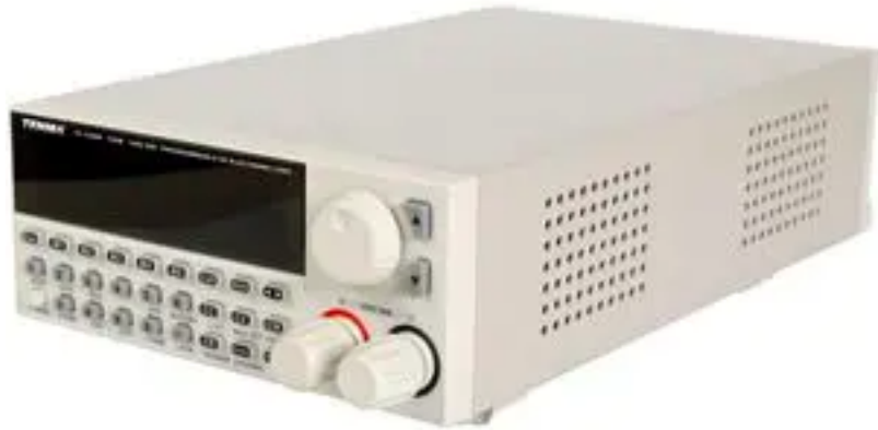
Figure 4.6: Electronic load used for discharging the batteries. Figure taken from [66].
