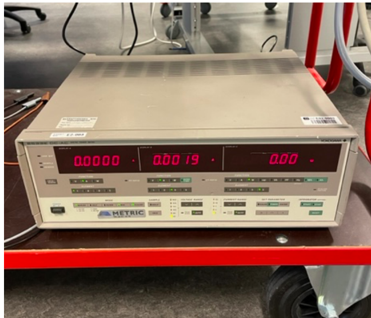
Figure 4.5: Digital power meter used for reading values for current, voltage and power.
