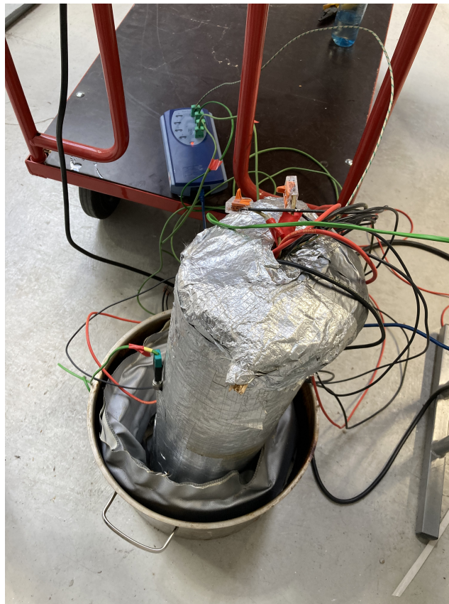
Figure 4.15: The dump load used for diversion during experimental work.
