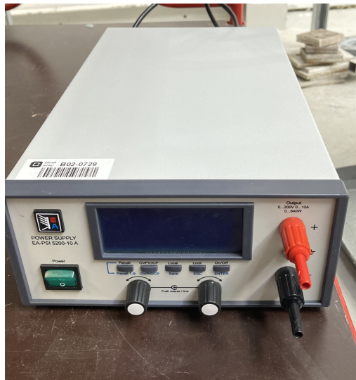
Figure 4.14: DC bench power supply used to test the system in diversion mode.
