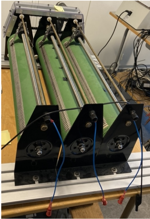
Figure 4.12: Three-phased rheostat used for varying the resistance in the system circuit.
