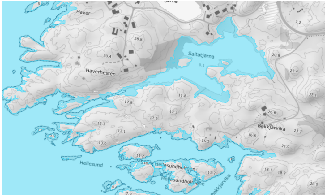
Figure 9: A projection of how a 200 year flood will affect the study area in 90 years (Norges Geologiske Undersøkelse, 2023b).
