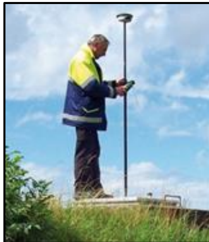
Figur 27: Rover/basestasjon ( Accurate GNSS Everywhere with SmartNet , u.å.).
