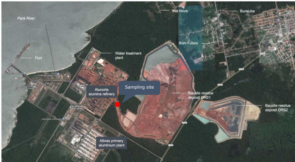
Figure 1-1 Hydro's Barcarena site layout. Rainwater that collects on BRDA is channeled to the edges, drained, and treated at the water treatment plant before being discharged into the Pará river. The red circles show the site of the samples used in this study. DRS and BRDA can be used interchangeably. From (Hydro, 2019).
