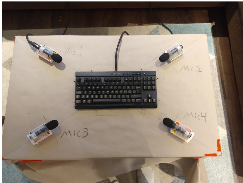
Figure 3.2: Physical setup with the keyboard in the typing position
