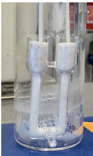
Figure 3.8: Crushed \text{NaAlCl}_4 blended with \text{NaCl} and \text{KCl} in the quartz cell.
