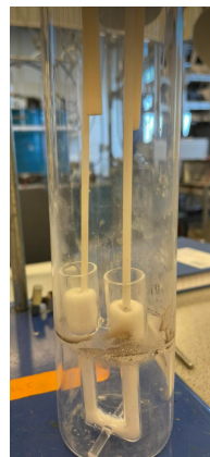
Figure 3.6: The setup of the customised cell inside the quartz crucible. The electrodes are covered in salt.
