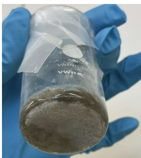
Figure 4.12: The product obtained after melting 50-50 mol% \text{NaCl-AlCl}_3 to a homogeneous mixture at 170 °C.
