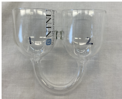
(b) The prefabricated cell.
