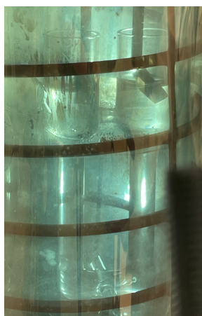
Figure 4.5: The quartz cell containing molten NaCl-KCl with eutectic composition inside the furnace.
