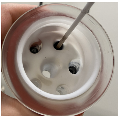
Figure 4.11: White coating seen inside the top of the crucible after the experiment.
