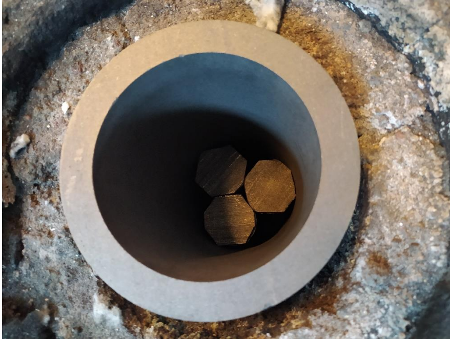
Figure 3.7: 3 samples are placed in smaller crucibles which were then placed in a larger crucible before beginning the melting process.
