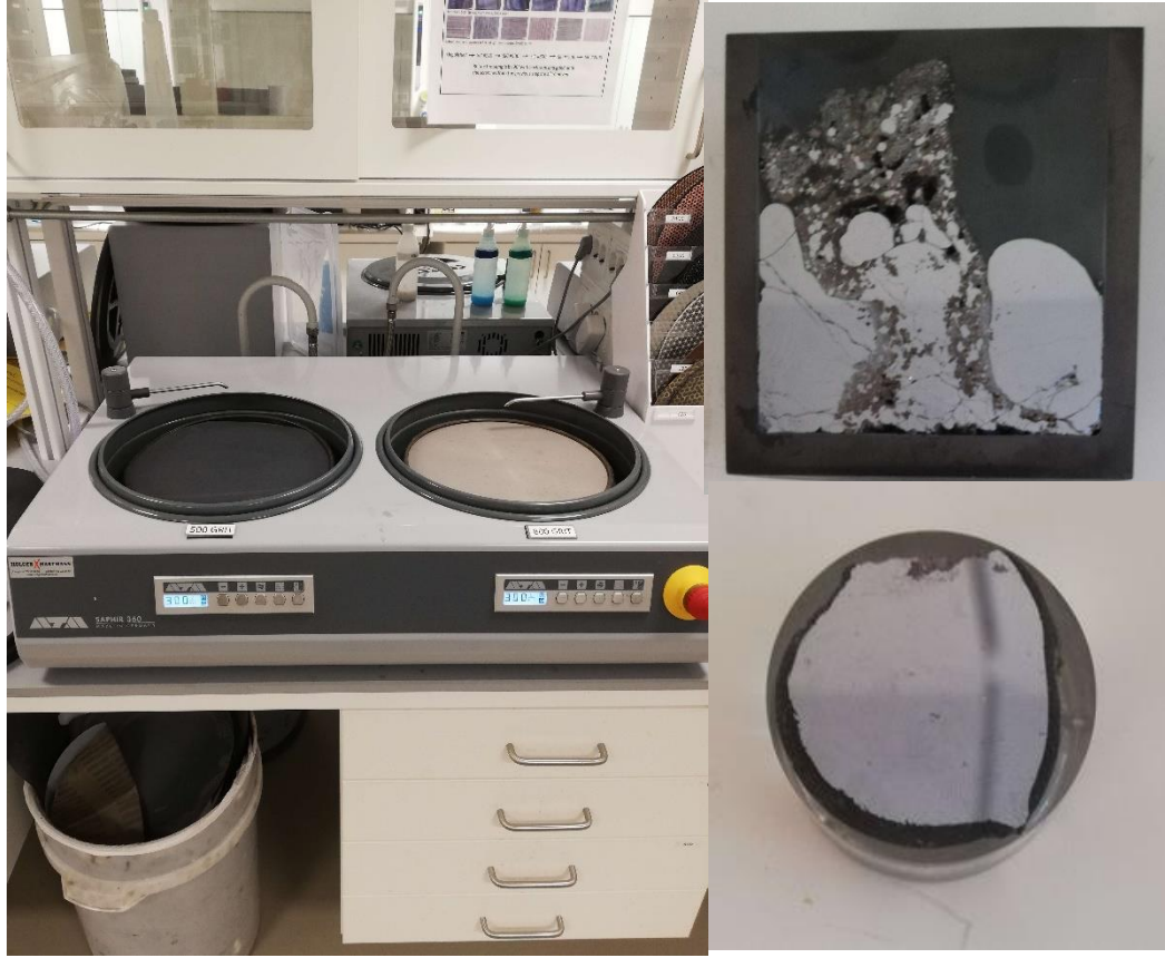
Figure 3.9: The Struers LaboPol-21 that was used for polishing along with the 2 different types of test samples that were polished.
