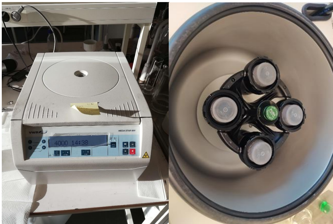
Figure 3.5: The VWR Megastar 600 centrifuge used to separate the silicon kerf sludge.
