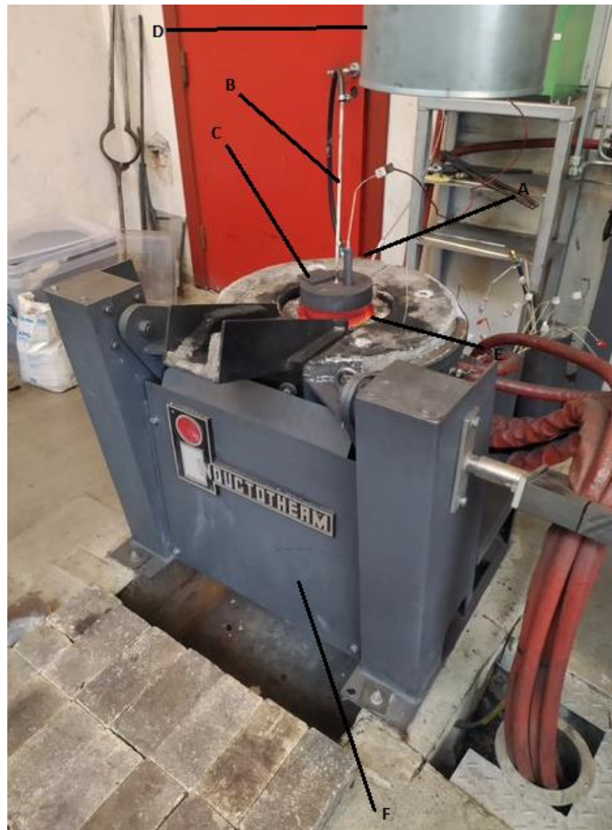
Figure 3.8: The IF75 induction furnace used to melt the silicon kerf. A points towards the thermocouple, B points towards the argon gas tube, C points towards the covered lid hole, D points towards the ventilation tube, E points towards the main graphite crucible and F points towards the furnace body.
