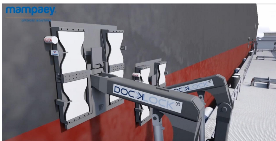
Figur 2.2: Dock Lock magnetisk fortøyningsystem (Bilde). Mampaey - https://unece.org/DAM/trans/doc/2013/dgwp15ac2/Dock_lock_presentation_1.pdf (Hentet: 02.04.2023).
