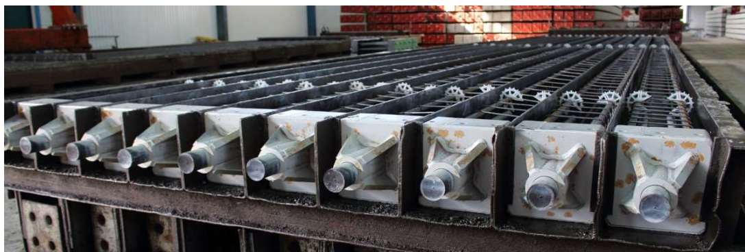
Figur 4: Betongpeler i form (Nor-pel, u.å.)
