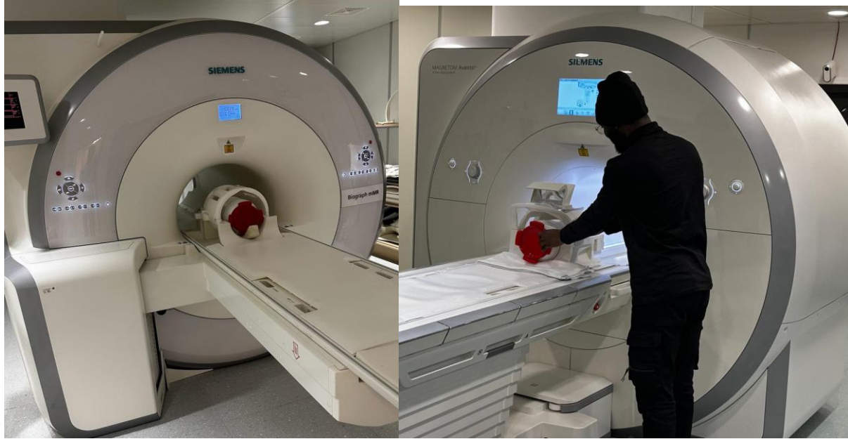
Figure 3.2 (a) Image of 3T Siemens Biograph mMR (b) Image of 1.5T Siemens - MAGNETOM Avanto fit, both with set up of the new phantom. The images were taken at St Olavs Hospital.
