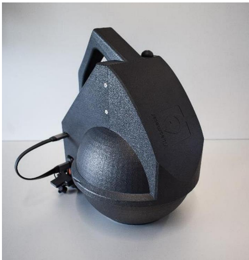
Figure 1-6 The VideometerLite multispectral imaging prototype (Schultz et al., 2023).
