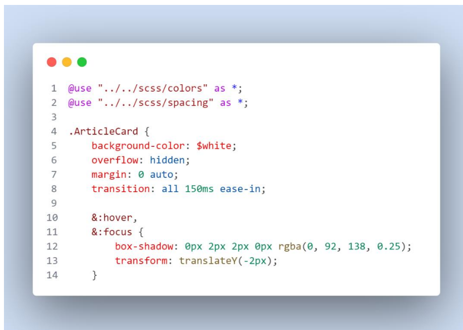
Figure 12 – Example of how a component is styled: Every element is styled and nested inside ".ArticleCard" className, and color and spacing variables are imported in the file
