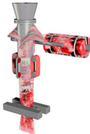
Figure 8: Illustration VFFS machine [21]
