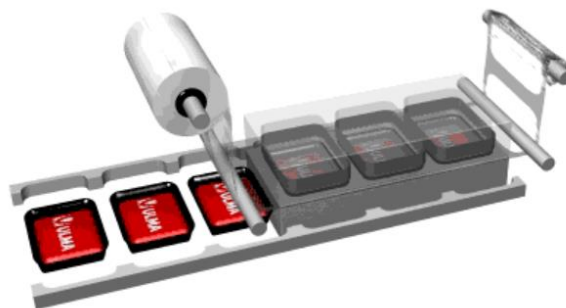
Figure 10: Illustration traysealers machine [26]
