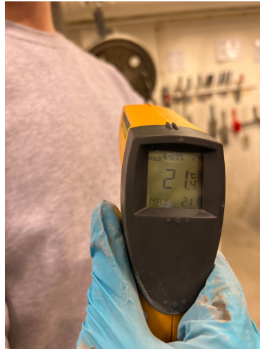
Figure 3.3.1: Infrared thermometer used for measuring temperature
