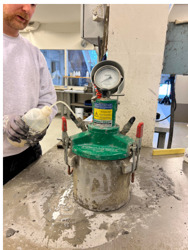
Figure 3.3.5: Measuring Air Content
