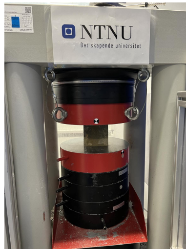
Figure 3.4.1: Toni TROL II, Model 0560 performing compressive strength test
