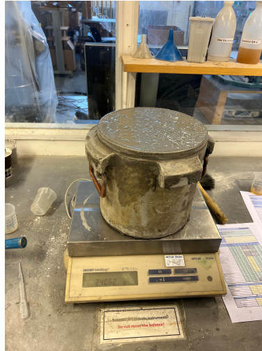
Figure 3.3.4: Measuring weight of fresh concrete in a 7983cm 2 container
