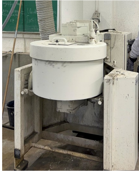
Figure 3.2.5: PMat Zyklos 50L Concrete tumbler
