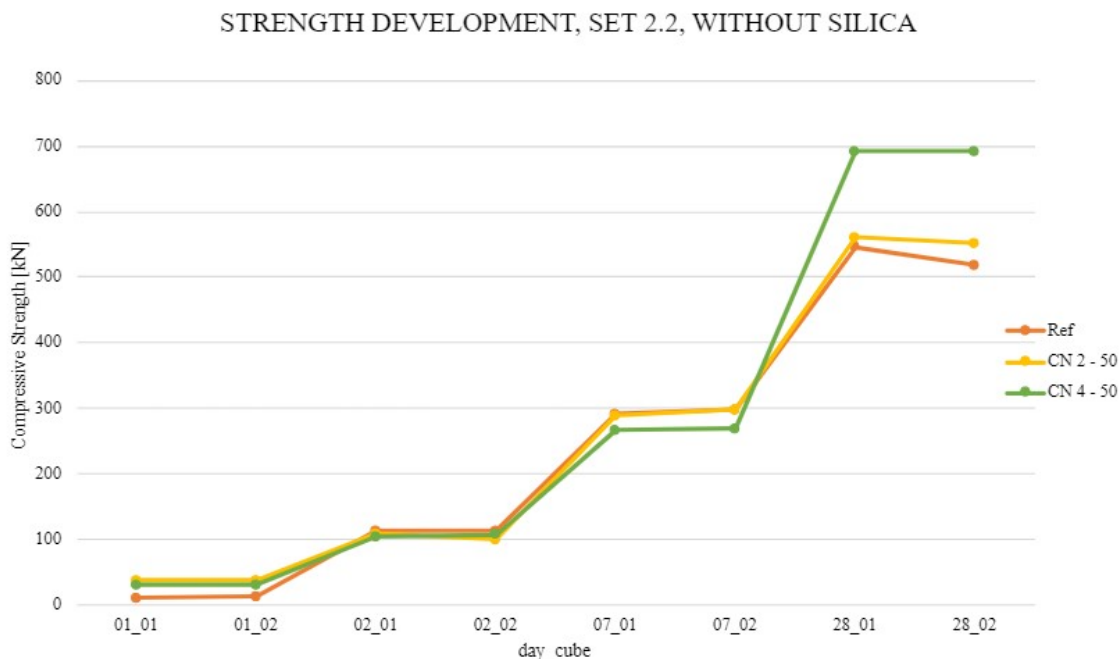
Figure 4.2.2: Set 2.2: Compressive Strength
