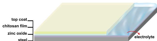
Figure 2. Representation of the layer composition of the sample used for delamination studies by SKP measurements. At the defect site, a solution of 5% NaCl was added to initiate cathodic delamination.
