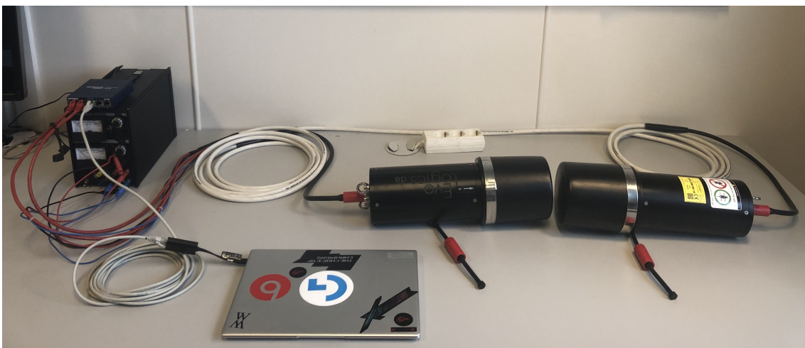
Figure 24: Image of the setup for the communication test in air with EvoLogics modem.
