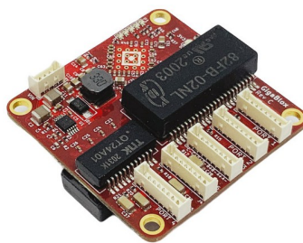
Figure 3.11: GigaBlox Ethernet switch.
