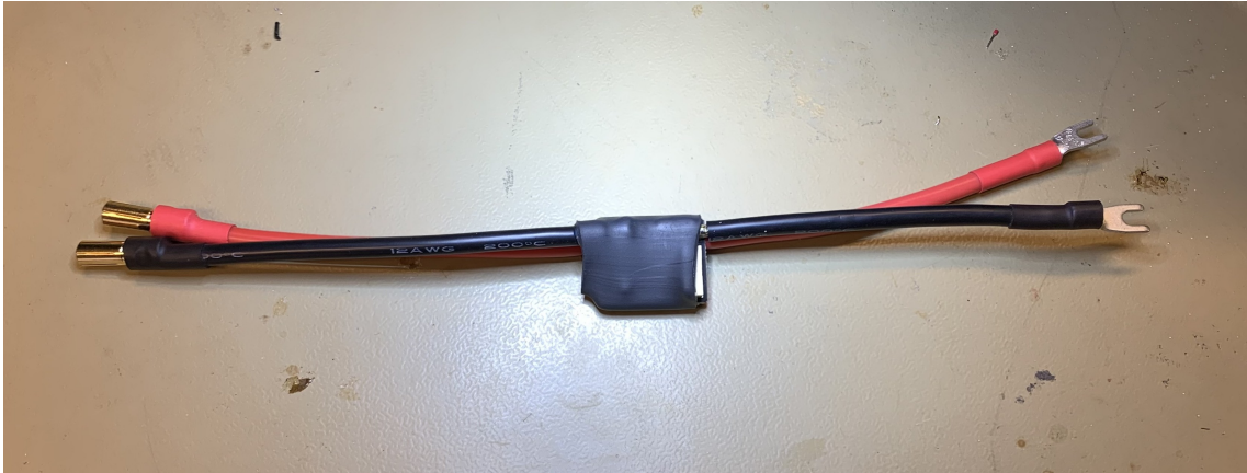
Figure 6.14: PSM with the soldered ground and new heat shrink.
