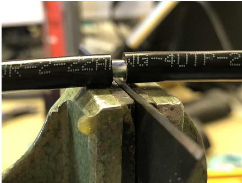
Figure 5.2: Cable stripping with a blade mounted to a table vise.
