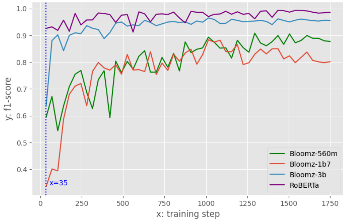
Figure 7.11: F1-scores measured every 0.02 epochs over one epoch of training on the CRA-dataset with batch-size=8 (meaning 8 datapoints every training step).
