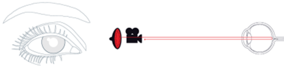
Figure 6: Image portraying the bright pupil effect, with the camera and light being in line with each other.
