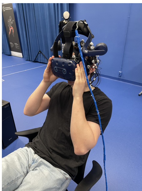
Figure 40: An image showing how a participant would wear the equipment when testing the speller.
