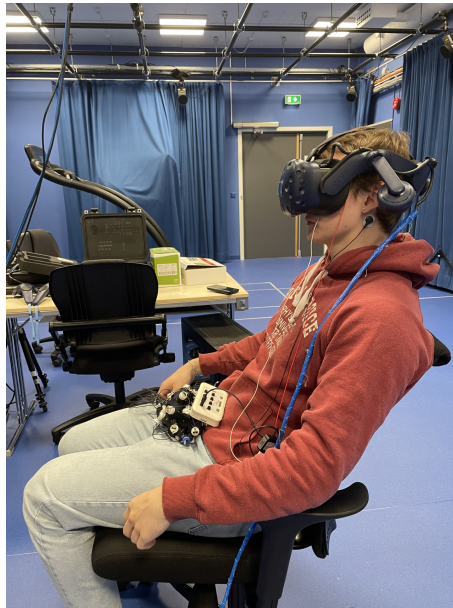
Figure 26: The figure shows how the equipment was put on the group member used to generate blinking data. Here you can see the member having the EEG in his lap and the EMG by the left eye, with the VR headset containing the eye tracker also equipped.
