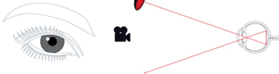
Figure 7: Image portraying the dark pupil system, with the camera and light off axis.
