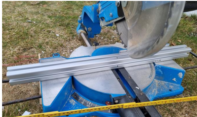
Figure 47 Cutting aluminium profile with miter saw.
