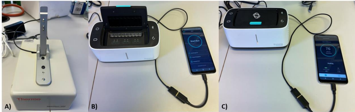
Figure 4: A) nanodrop 100 spectrophotometer used for measuring nucleic acid (DNA) concentration. B, C) Biomeme Franklin qPCR. B) setup in the qPCR with samples, C) qPCR running, each round of samples had a 76 min laps with conditions after Tarrant et al. (2008).
