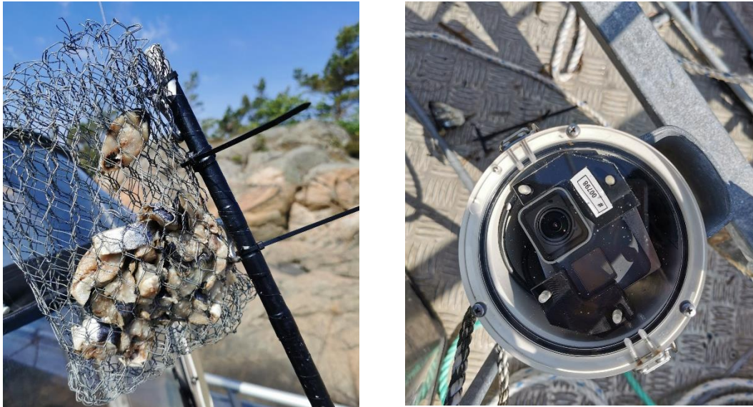
Figure 4: Stereo-BRUV details. (a) Chopped up herring was used as bait. (b) Go-pro cameras were used in this stereo-BRUV setup. Photo: Astrid Winnberg Skoge.
