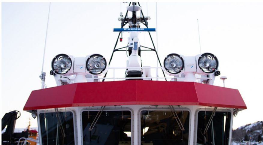
Figure 1.1.1: Two CL-38 mounted on a ship's bridge
