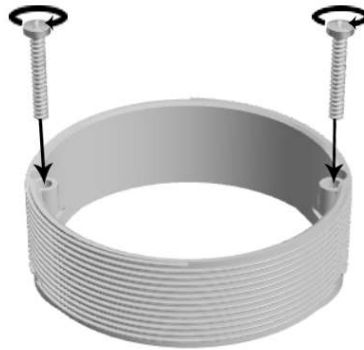
Figure 1.3: Inserting screws into adjustment rings
