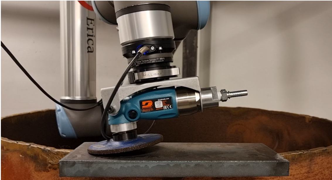
Figure 28: Setup for first grinding tests (safety guard removed for illustrative purposes)
