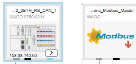
(a) Wago PLC and Modbus
