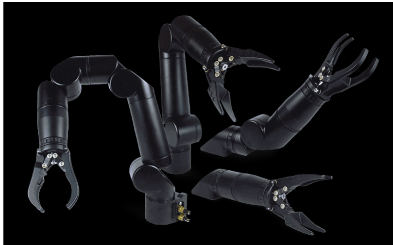
Figur 10: Reach Bravo Mk2, robotarm designet for maritimt miljø (ReachRobotics, 2023)
