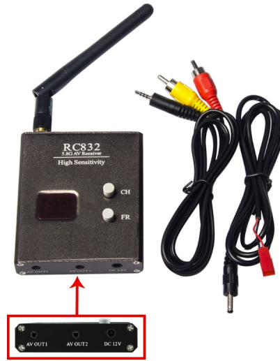
Figure 28: Receiver pin layout and AV/MiniJack cable
