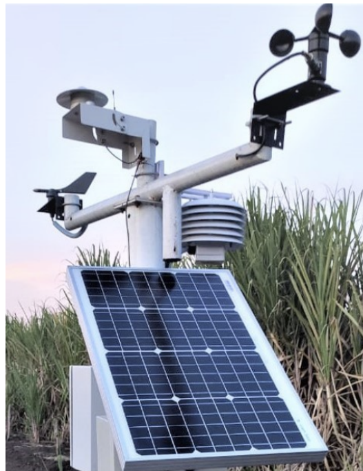
Figure 2.5: PV panel aligned with the weather station tree.
