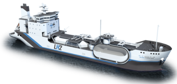
Figure 3.7: Suiso Frontier, cryogenic hydrogen carrier ship[68]
