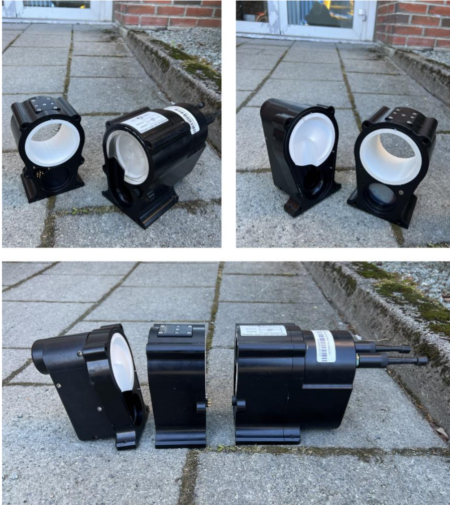
Figure 2.3 The UBAT separate, clearly showing the detection chamber where bioluminescence is emitted. Both impellers are out but would normally be put in the middle part of the UBAT underneath the detection chamber. Photos: Gitte Krohn-Pettersen.
