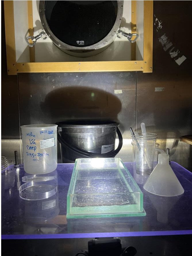
Figure 2.5 Showing the set up for sorting on board G.O. SARS. It was easier to have the room dark with minimal light from light sources above during sorting. Photo: Gitte Krohn-Pettersen
