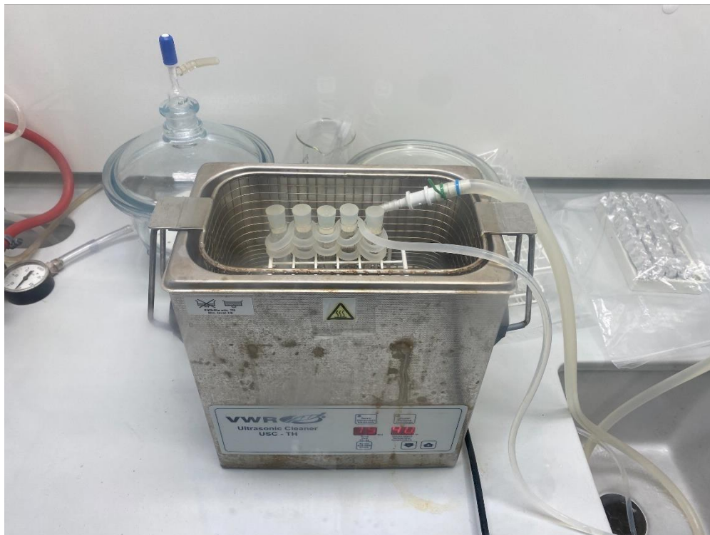
Figure 16. The "mini-soxhlet" in action. The silicone tubes are attached to the cold water faucet to the right. Photo by Author.
