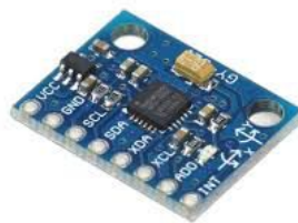
Figure 3.3. MPU-6050 6-DoF accelerometer and gyroscope, reprinted from [14].
