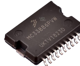
(b) MC33886PVW motor driver, adapted from [12].
