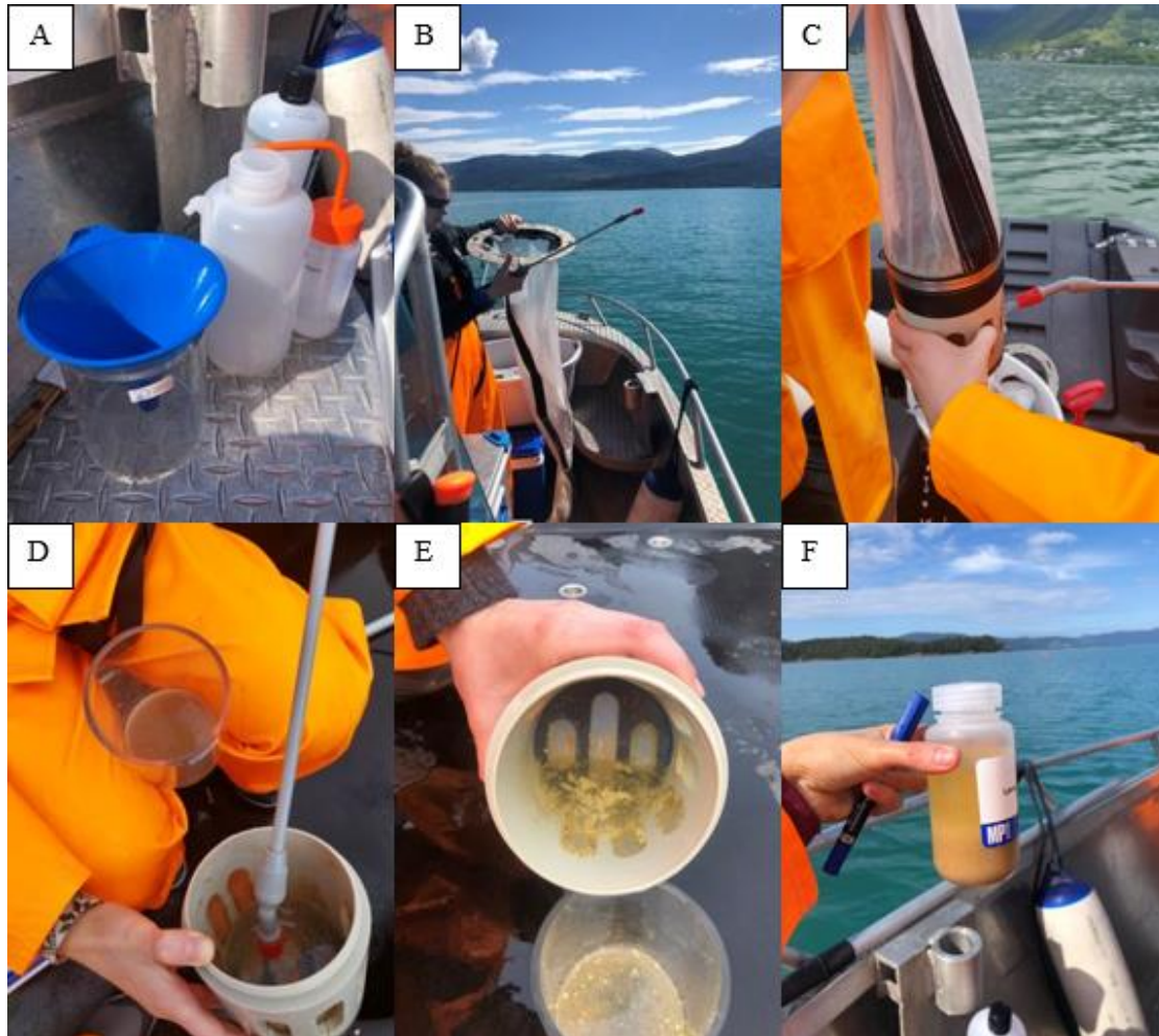
Figure 7: Plankton processing in the field. A: The equipment used for plankton processing. Ethanol, spray bottle for ethanol, spray bottle for water, sieve, and funnel. B: Rinsing down the plankton net with saltwater before taking the collection cup of. C: Spraying down the cup from the outside to get as much of the plankton growth of the mech net before taking the cup off. D: Rinsing out plankton out of the collection cup into the sieve using saltwater. Photo: Amanda Andersson. E: Plankton sample before rinsing it over into the sieve. F: Finished sample ready for storage. Pictures: Amanda Andersson/Ingvild Tryggestad.
