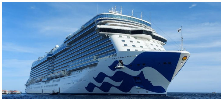
Figure 5.1: A raked and flared bow. This ship has a bulb as it is unusual for ships not to.
