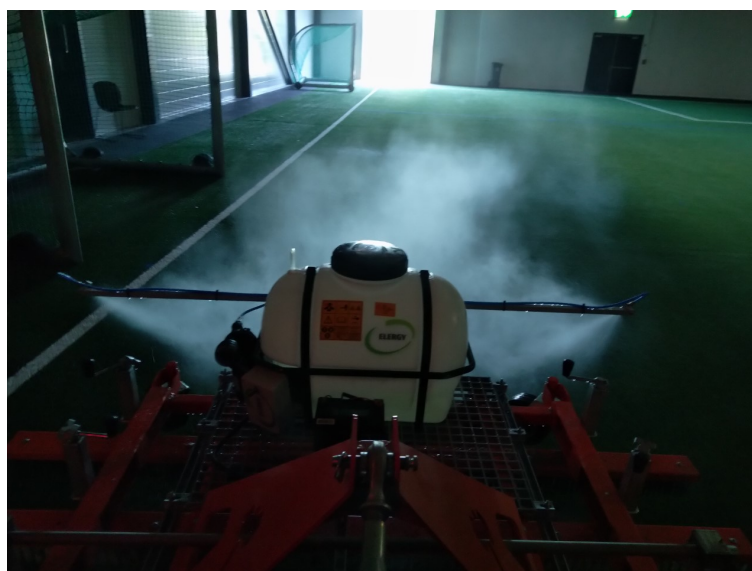
Figure 2.3: An in action picture of the disinfection device used to apply Nüscosept PRO to the indoor artificial turf at Flatåshallen.
