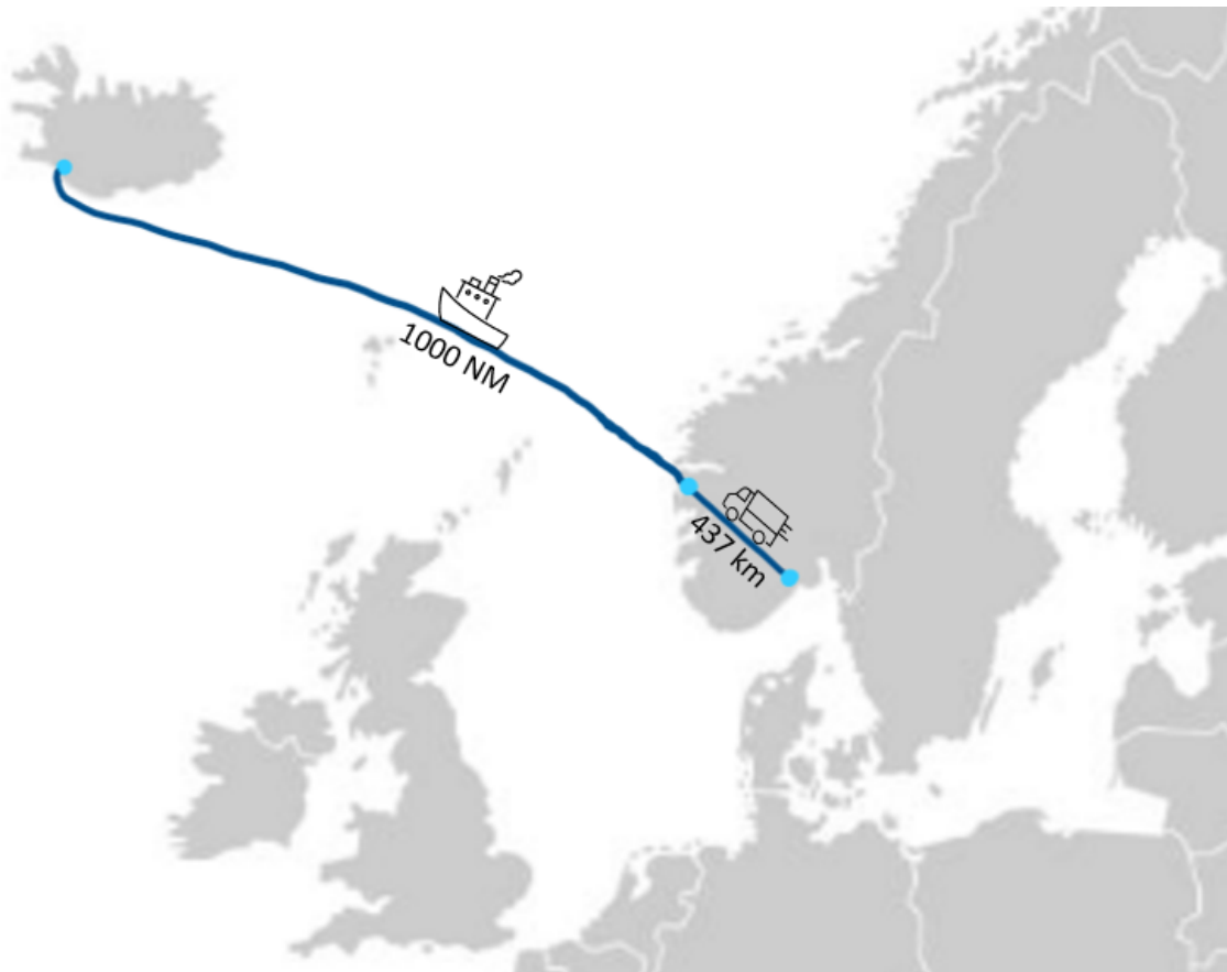
Figure 4.3: Ammonia is transported by truck from Porsgrunn to Mongstad, both in Norway. All three fuels are utilized in a oil/chemical tanker from the delivery site in Mongstad to Reykjavik, Iceland.
