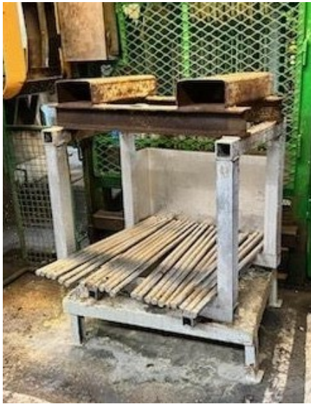
Figure 4.3.2: Currently the rods are stored and transported in these containers.
