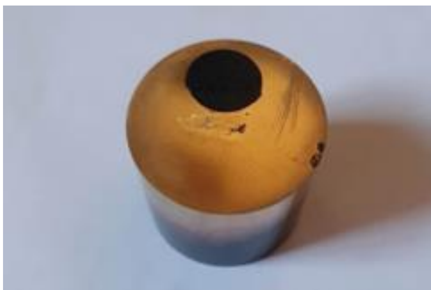
Figure 3.7: Shows sample 1 prepared for SEM, molded and coated.
