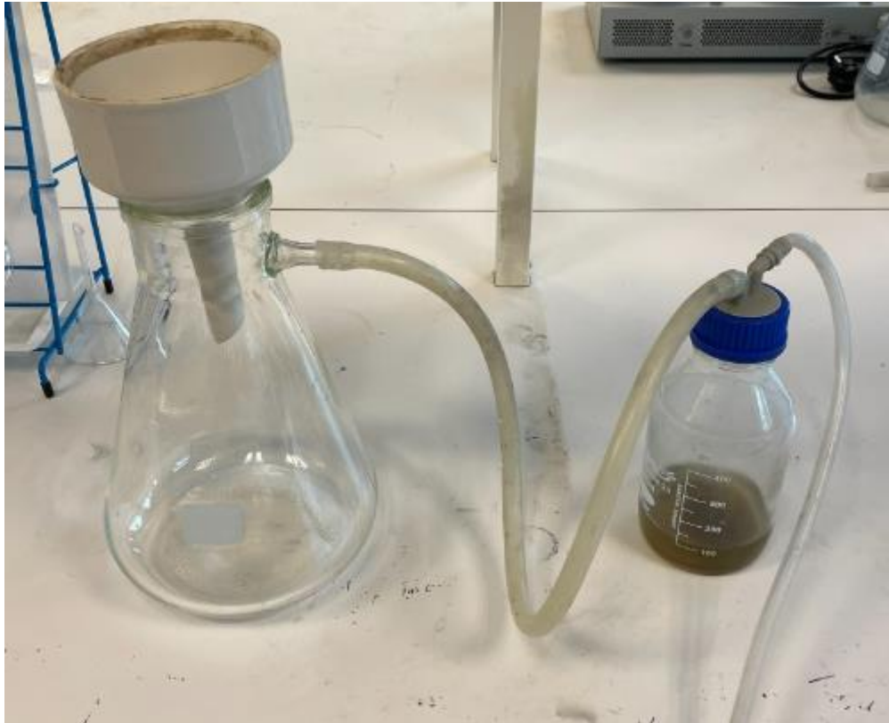
Figure 3.6: Filtration setup for separation of solid residues from solutions.
