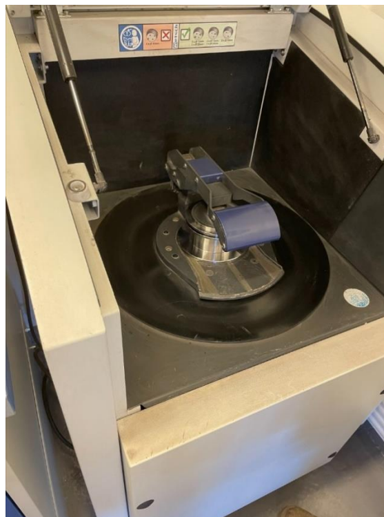
Figure 3.4: Shows the milling machine with sample placed inside.
