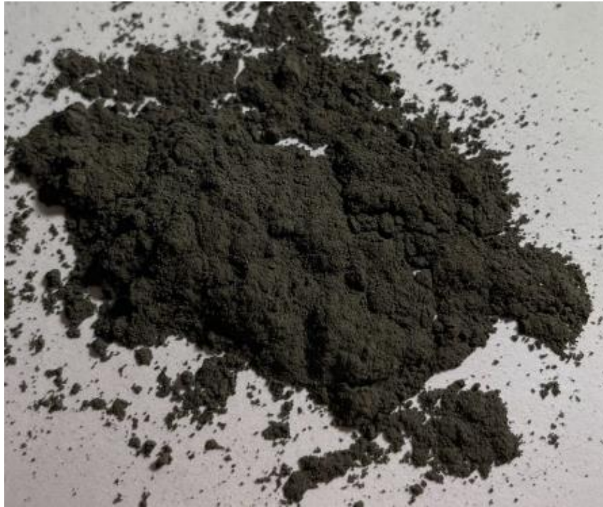
Figure 3.5: Reduced ore after milling to <60 microns.
