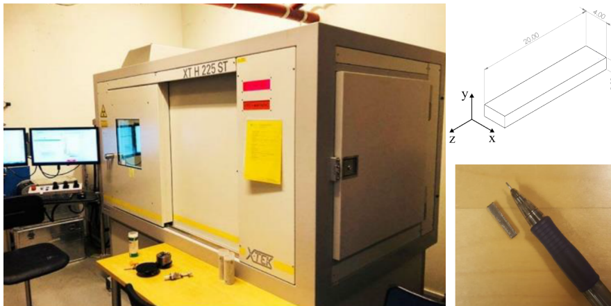
Figure 3.6: XCT machine and geometry of the specimen investigated. Measures are given in mm.
