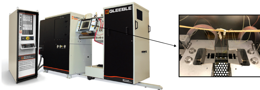
Figure 3.26: Gleeble GTC 3800 with sealing chamber for vacuum and inert environment
