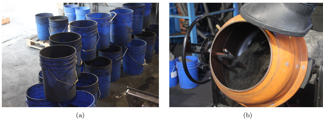
Figure 3.3: Weighing and mixing of raw materials. Materials weighed out in separate buckets (a), and cement mixer with charge (b)
