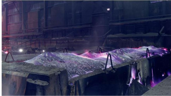
Figure 2.6: A movable furnace from the Volga abrasive plant, ready to be fired [37].
