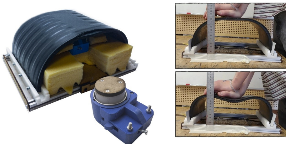
Figure 3.2 P1 Prototype of a chest with rib fracturing haptics device for CPR training. On the right demonstration and testing of deforming the chest structure by compressions is shown.
