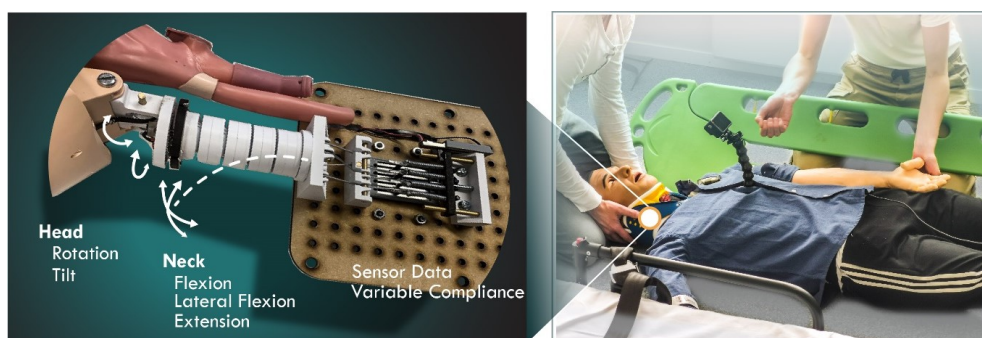
Figure 3.6 P5 Prototype of the neck concept. The testing setup with the concept integrated in a modified simulator shown on the right.
