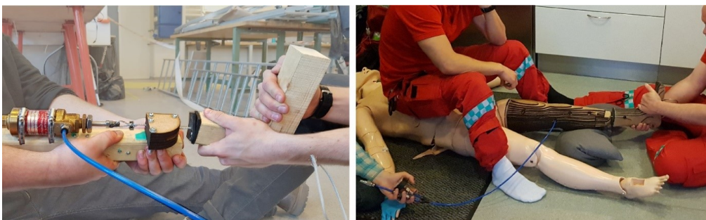
Figure 3.3 P2 Prototypes of a fractured leg task trainer. On the left, functional prototype using pneumatic cylinder and simple topology. On the right, a higher fidelity prototype (using the pneumatic system), integrated with an existing simulator for paramedics to test.
