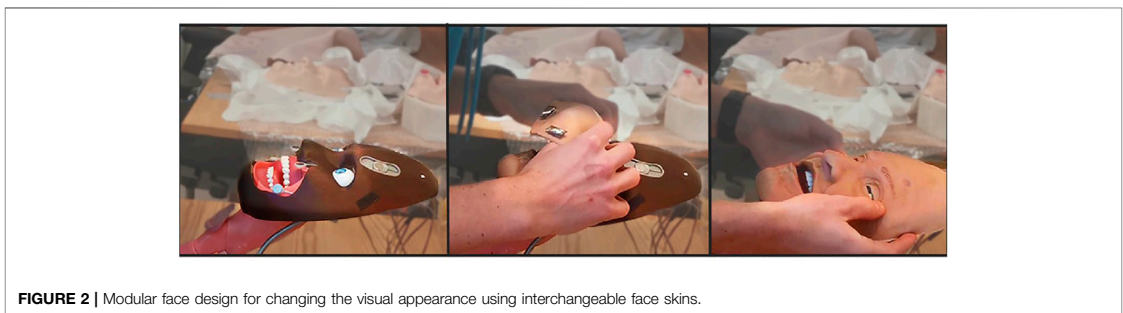
FIGURE 2 | Modular face design for changing the visual appearance using interchangeable face skins.
