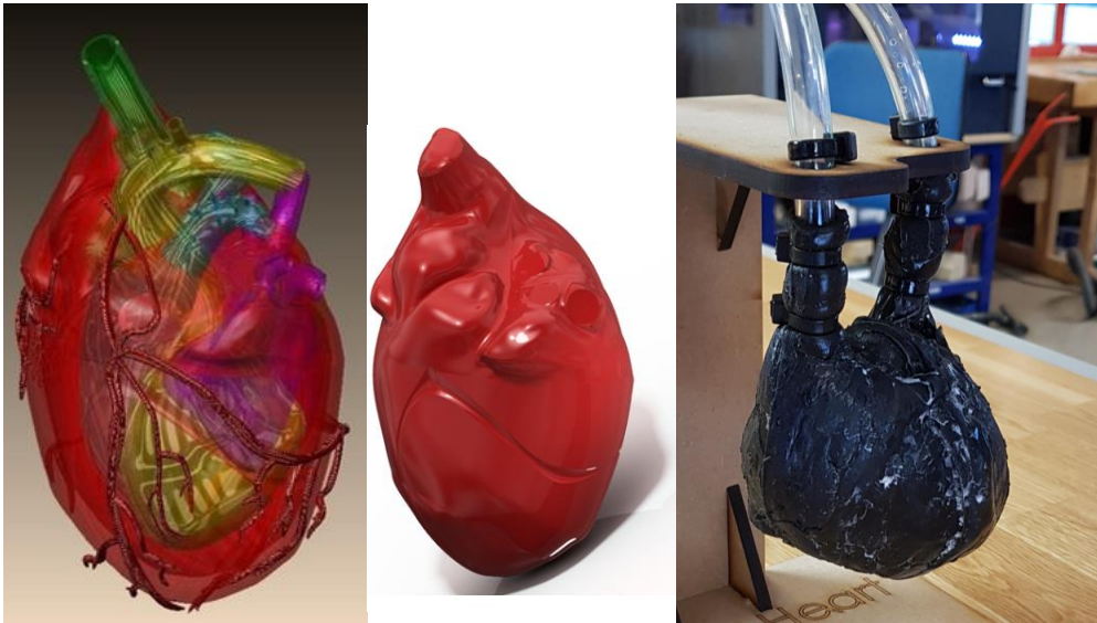
Figure 5. A human heart represented by a virtual prototype (left and centre) and a physical phantom (right) built using moulding with flexible materials
