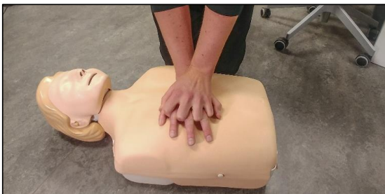
Fig. 1. Example of one commercially available resuscitation mannequin. This uses a linear compression spring mechanism to enable chest compressions.
