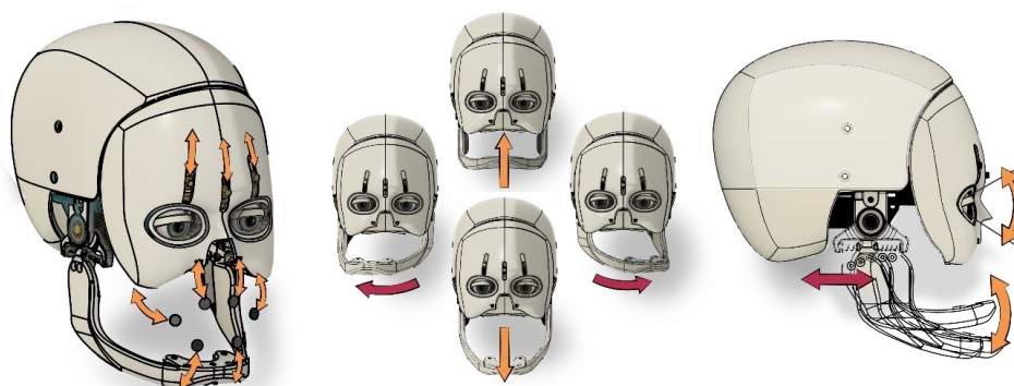
Figure 3.11 The mechanical design of the simulator face concept. Modes of actuation (orange) and passive compliance (red) are indicated with arrows.
