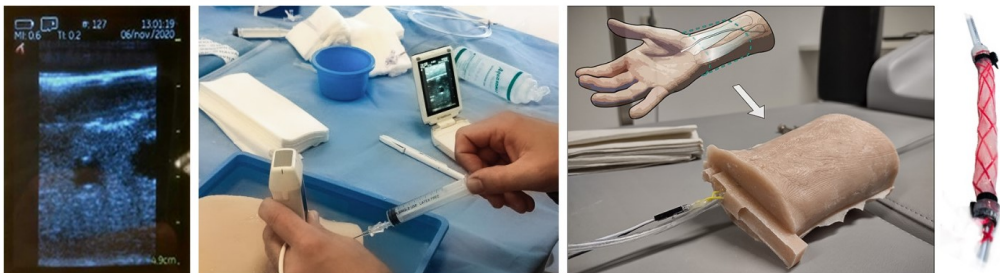
Figure 3.4 P3 Vascular phantom prototypes. From left an ultrasound image of the simulated artery and vein, medical professional using handheld ultrasound probe guiding a needle insertion, vascular wrist phantom, and the braided sensor.
