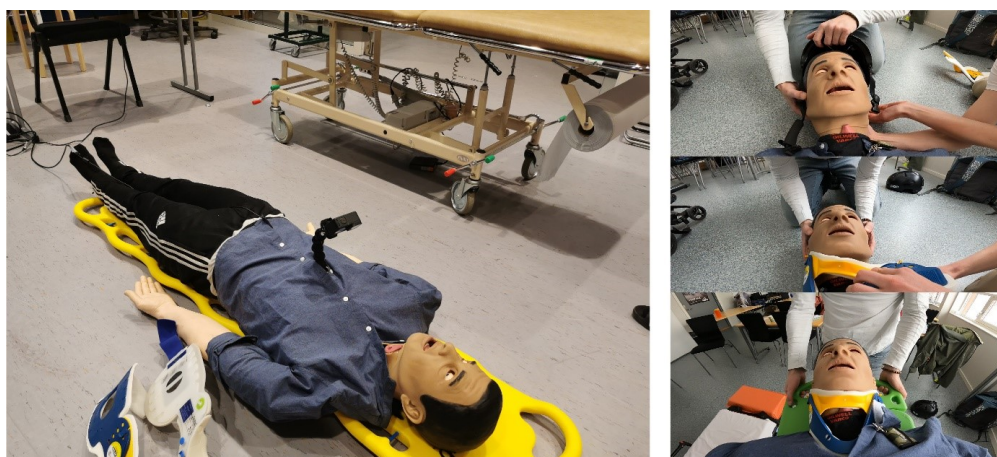
Figure 4.11 User testing of neck immobilization and patient transfer in P5.
