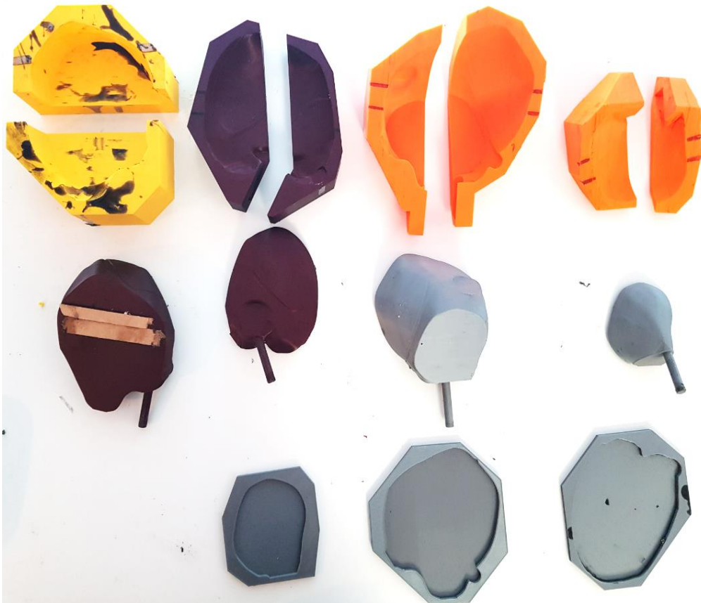
Figure 4. Mould negatives built using rigid materials that were used for moulding flexible phantom hearts with flexible material
