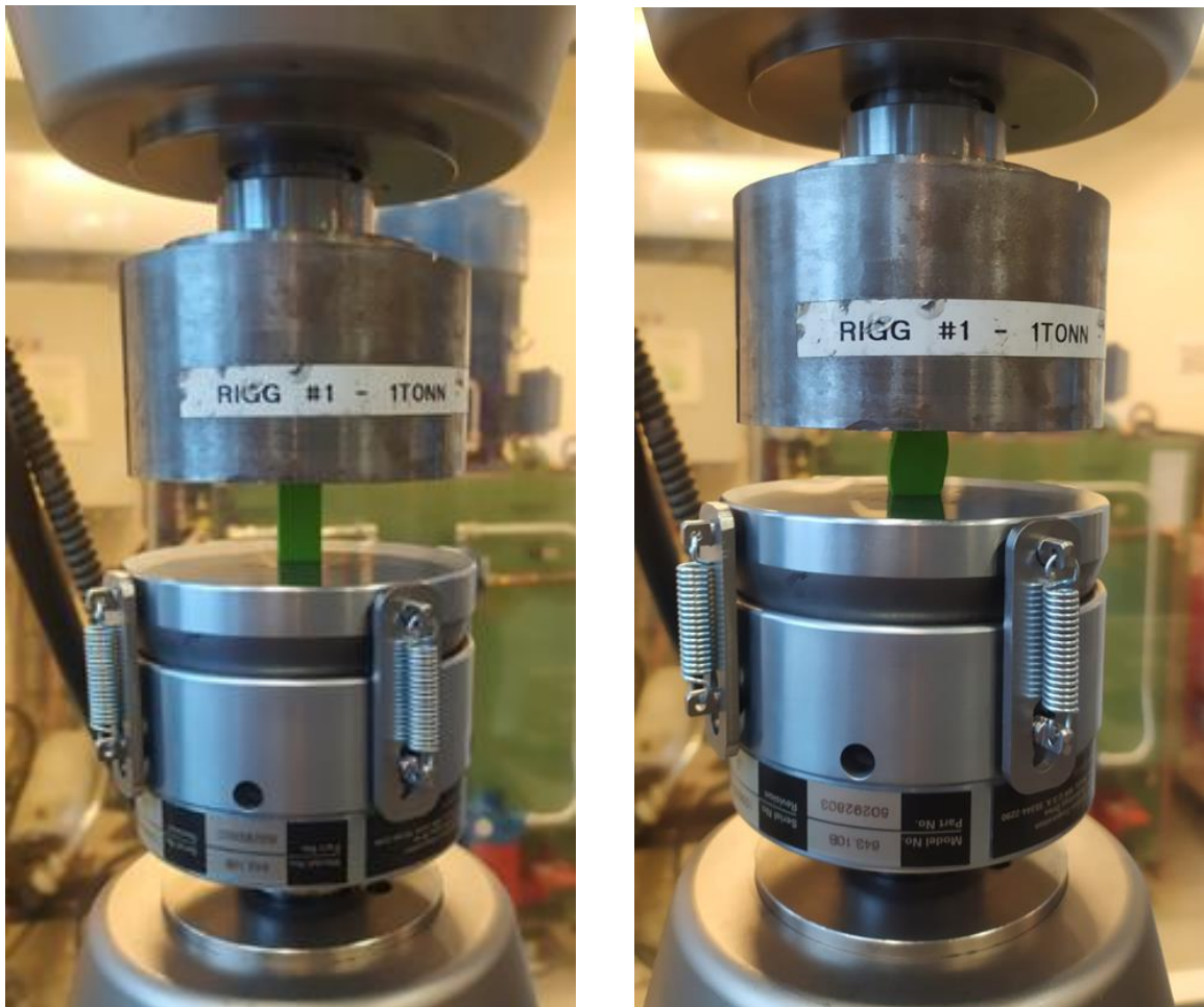
Fig. 3.18. on the left the PLA specimen prior the compressive test and on the right the PLA specimen after the compressive test was performed.
