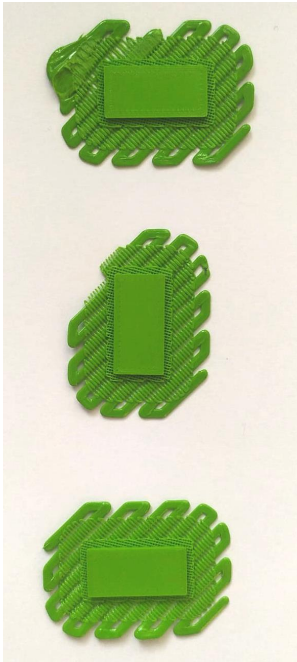
Fig. 3.6. on top the specimen printed with an angle of 0^\circ ; on the center the specimen printed with an angle of 90^\circ , at the bottom the specimen printed with an angle of 45^\circ . The specimen outlines some damage that is not related to the printing process.
