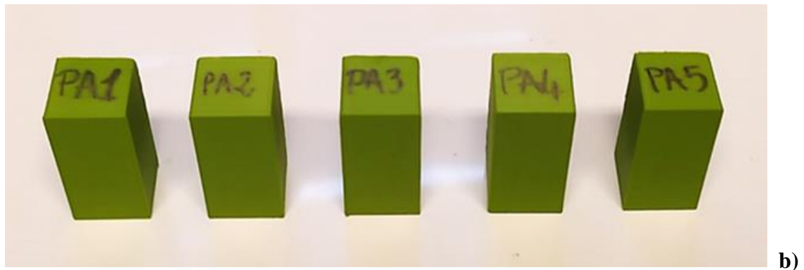
Fig. 3.1. (a) specimen still attached to the raft; (b) the five specimens used for the compressive test.
